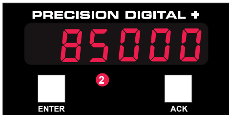
PD690 indicating that Alarm #2 is in alarm condition.
